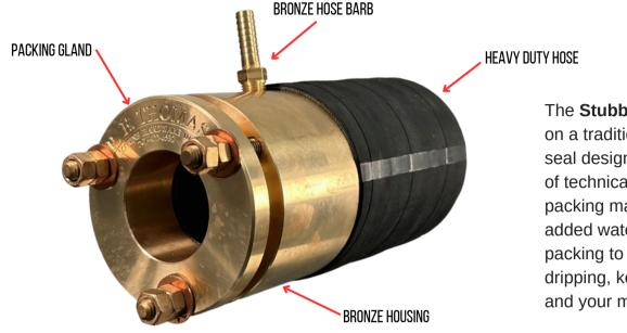
The **Stubby Pro** is a modern take on a traditional self-aligning shaft seal designed to take advantage of technical advancements in packing material technology. The added water feed allows the packing to remain cool without dripping, keeping your bilge dry and your mind at ease.
